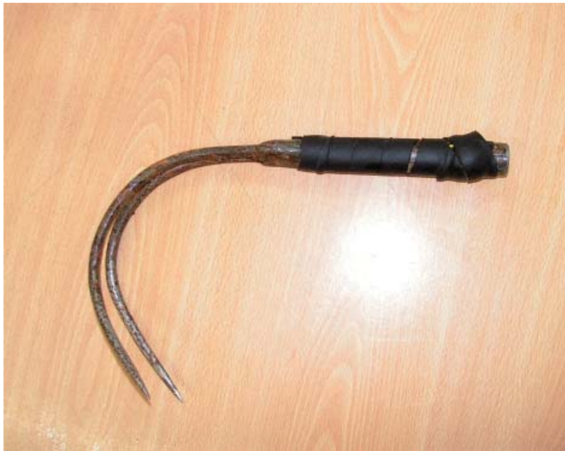
Figure 10. Double hook used in Chile for harvesting razor clams (Photo credit: Irene L pez G., Daniel Arriagada O. and Flor V jar D.).
