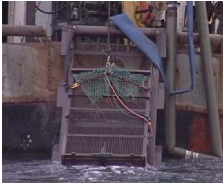
Figure 13. Hydraulic dredge for razor clam.
