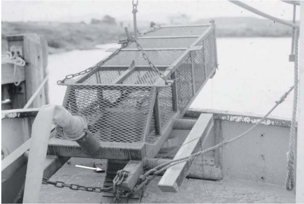
Plate 1. View of a typical hydraulic blade dredge used in parts of Scotland in the period 1988-2003. View is from the front of the dredge and shows the layflat hose and manifold used to deliver water from the deck pump. Image also shows stabilising runners on the sides of the dredge and the mesh of the collecting cage. The hollow blade or ‘tooth’ can just be seen on the underside of the dredge (arrowed).
