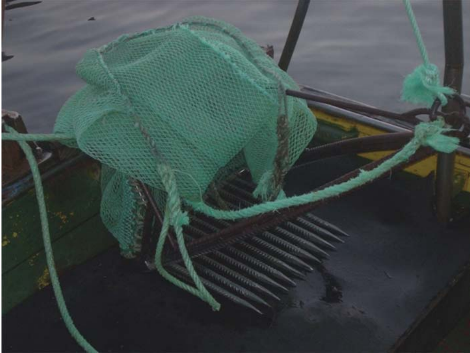
Figure 12. Portuguese razor clam dredge (Photo credit: Miguel B. Gaspar).
