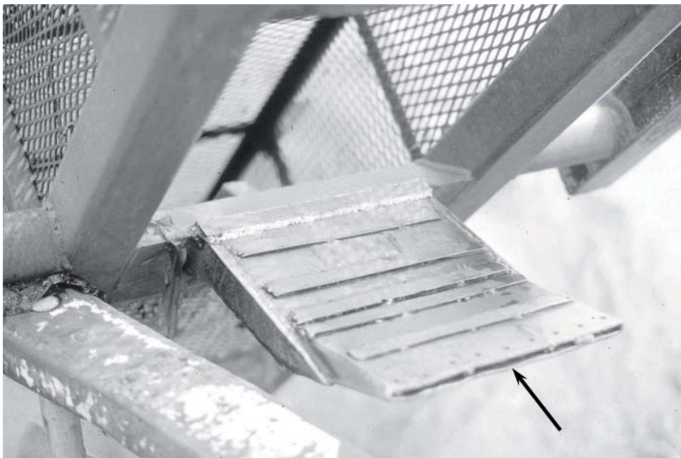
Plate 2. View of the box section blade or ‘tooth’ of the hydraulic dredge used in parts of Scotland in the period 1988-2003 (as in Plate 1). Image shows the longitudinal taper and the 10 mm gap along the leading edge (arrowed). Image is taken of the underside of the dredge viewing the front face of the blade at an oblique angle.
