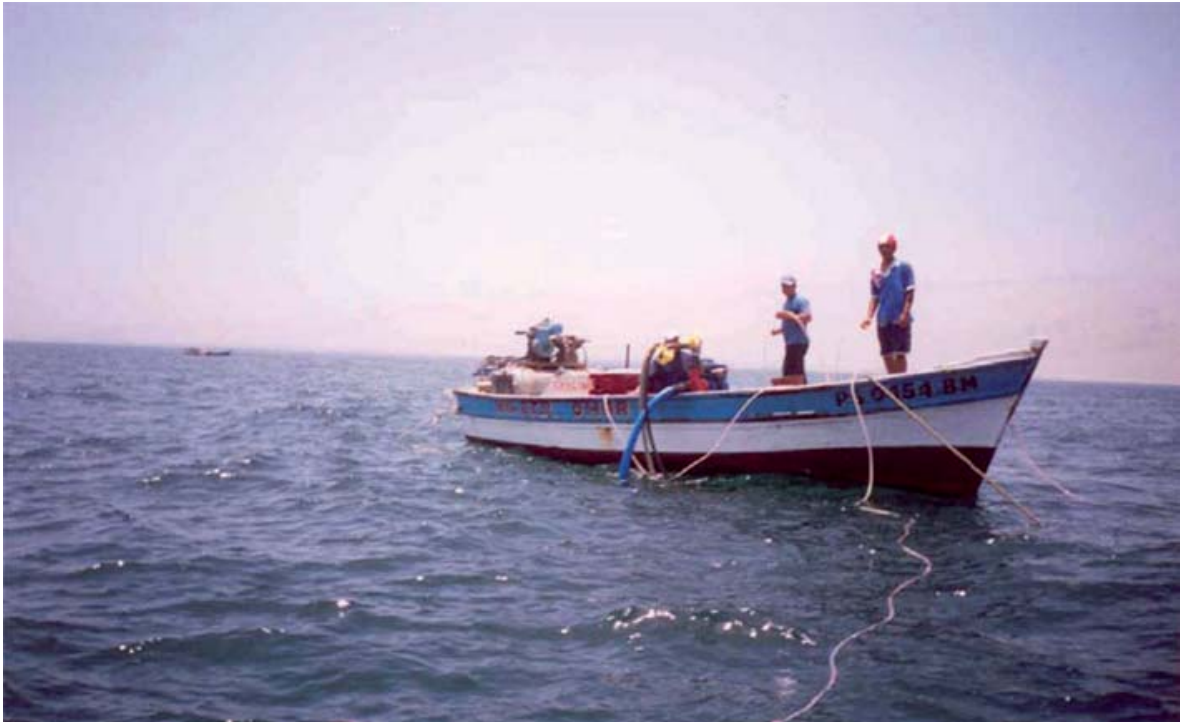
Figure 11. Artisanal fishing boat used in razor clam fishery in Peru, showing the deck equipment used to pump water at high pressure through a hose (Photo credit: Jaime Mendo and Roberto Espinoza).
